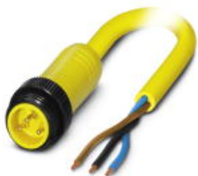
Power cable, 3-position, PVC, yellow, Plug straight 7/8"-16UNF, A - standard, on free cable end, cable length: 1 m
