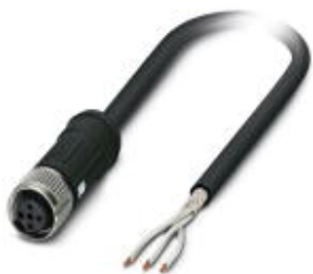
Sensor/Actuator cable, 3-position, PE-X halogen-free, black, shielded, free cable end, on Socket straight M12 SPEEDCON, A-coded, Cable length: 5 m, For railway applications
