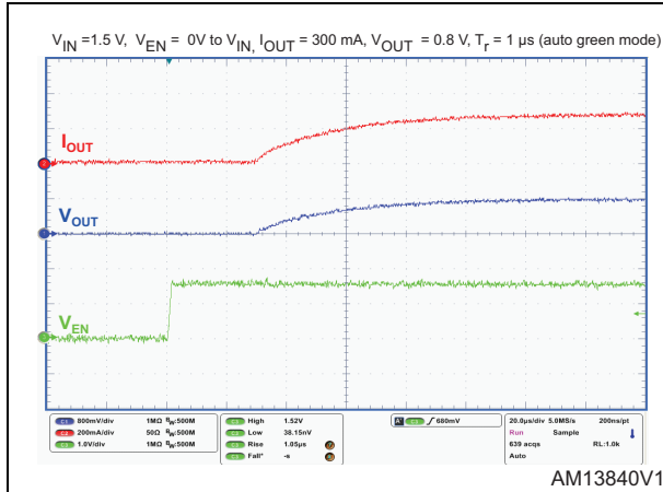
Figure 35. Startup by enable ( I_{OUT} = 300\text{ mA} , auto green mode)
