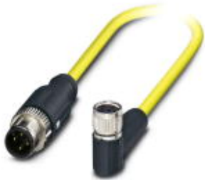
Sensor/Actuator cable, 4-position, PVC, yellow, shielded, Plug straight M12 SPEEDCON, A-coded, on Socket angled M8, Cable length: 1.5 m
