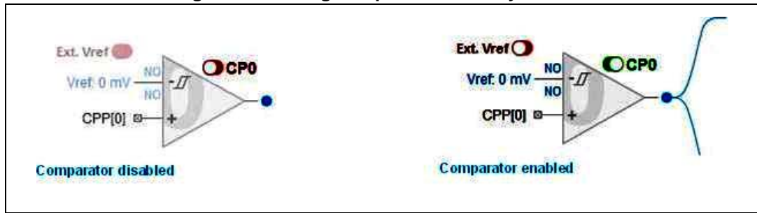
Figure 12. Analog comparators with hysteresis
