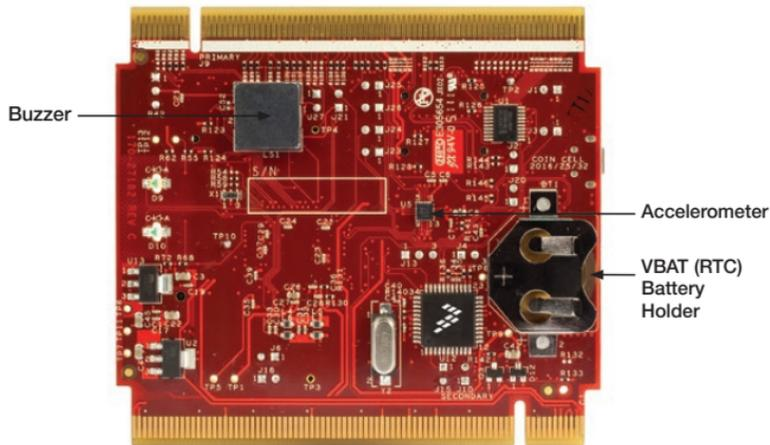
Figure 2: Back side of TWR-K20D72M board
