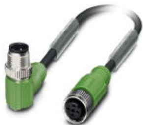
Sensor/actuator cable, 4-position, Variable cable type, shielded, Plug angled M12, A-coded, on Socket straight M12, A-coded, cable length: Free input (0.2 ... 40.0 m)
