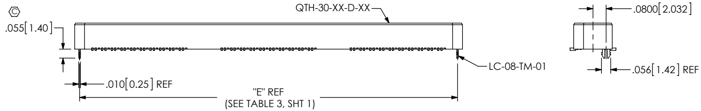
FIG 2 -LC: LOCKING CLIP OPTION (QTH-060-01-X-D-LC SHOWN) (DIFFERENT AS SHOWN, OTHERWISE SAME AS FIG 1)
