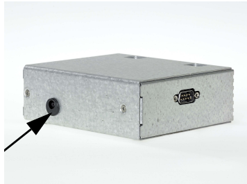
Figure 9-3 Low-voltage plug of the power supply unit
