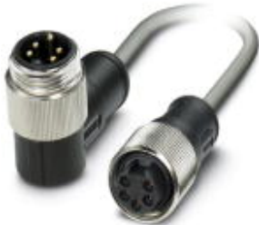
Bus system cable, DeviceNet, 5-position, PUR halogen-free, Gray RAL 7001, Plug angled 7/8"-16UNF, on Socket straight 7/8"-16UNF, Cable length: 10 m
