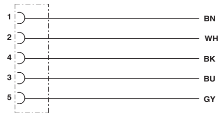
Contact assignment of the M12 socket
