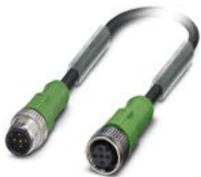
Sensor/actuator cable, 5-position, PUR halogen-free, black-gray RAL 7021, Plug straight M12, A-coded, on Socket straight M12, A-coded, cable length: 1.5 m
