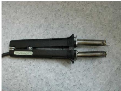
Figure 11. (Left) Thermal tweezers, Pace Thermotweez. (Right) Tool head, Pace 1121-0416-P1.
