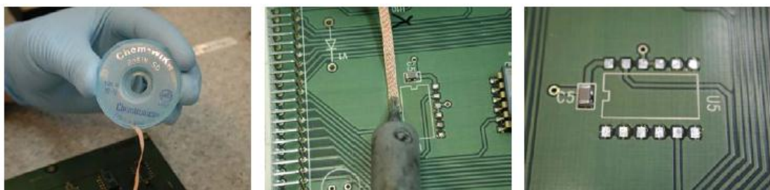
Figure 14. Soldering iron and solder braid used for solder removal.
