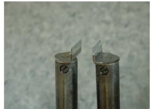
Figure 11. (Left) Thermal tweezers, Pace Thermotweez. (Right) Tool head, Pace 1121-0416-P1.
