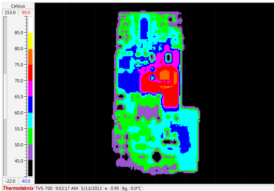
Figure 6. Thermal Map, Back Side at 24V IN and 10A OUT (T A = 25°C, 200LFM)
