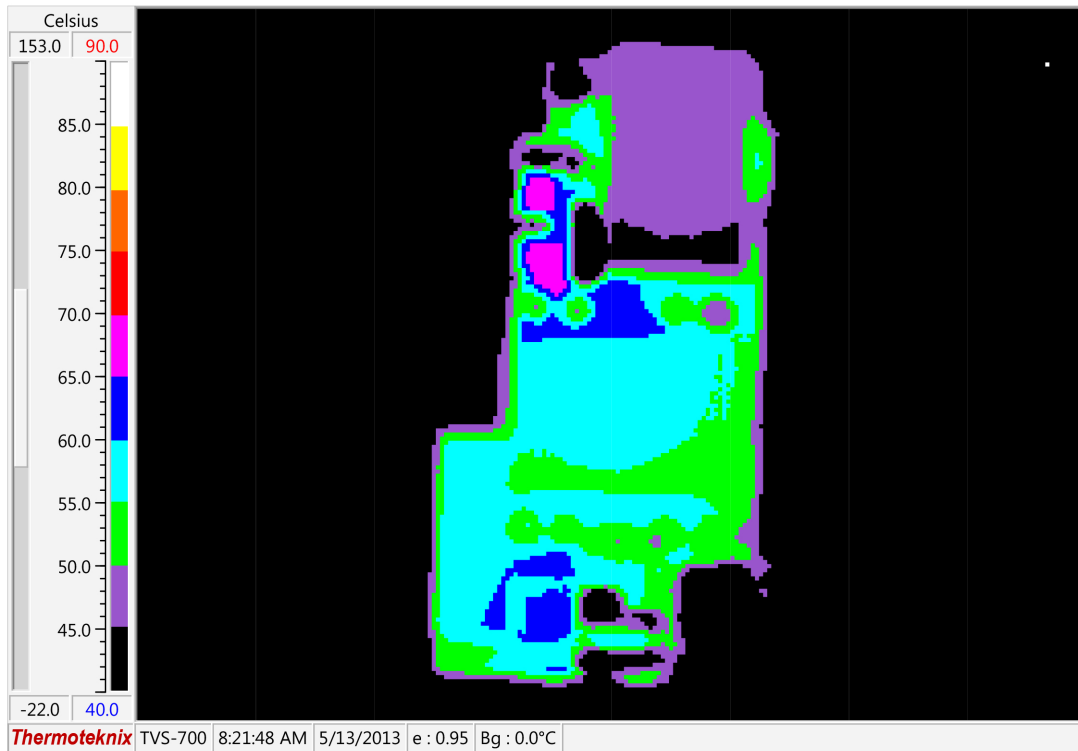
Figure 5. Thermal Map, Front Side at 24V IN and 10A OUT (T A = 25°C, 200LFM)
