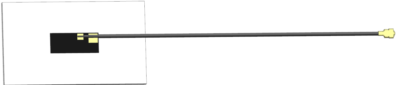
FIGURE4.1.1 ANTENNA LOADED WITH PC/ABS BLOCK OF 2MM THICKNESS
