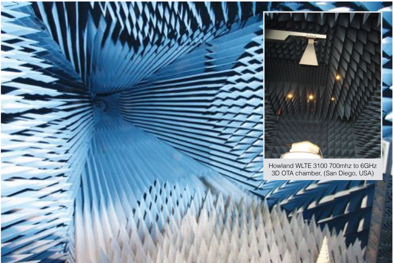
Taoglas' 12 metre 400 MHz to 6000 MHz ETS Lindgren 3D Tapered Anechoic Chamber in Wexford, Ireland
