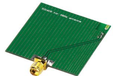
CAD.50 (Evaluation Board for CA.50)
