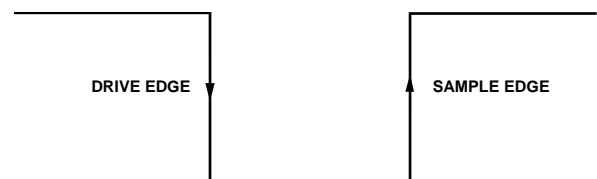
Figure 66. SPI Mode 3, SCLK Edges
