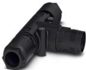
QUICKON T-distributor, black, 4+PE-pos., 2.5 mm 2 ... 6.0 mm 2 /690 V/40 A, for cable diameter of 12 mm ... 20 mm, with two QUICKON nuts
