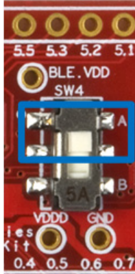
Figure 4-17. SW4 Position for Programming EZ-BLE
