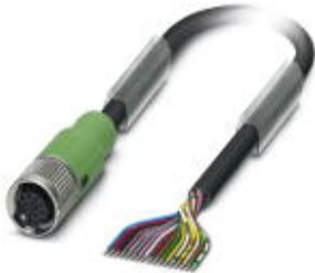
Sensor/Actuator cable, 17-position, PVC, Black RAL 9005, Free cable end, on Socket straight M12-SPEEDCON, A-coded, Cable length: 15 m
