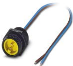
Flush-type connector, 2-position, Plug, straight, 7/8"-16UNF, on free cable end, Front mounting, with 1/2 inch-14 NPT mounting thread, Individual wires, cable length: 1 m
