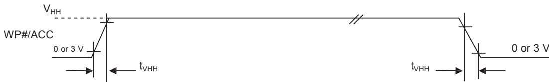
Figure 11. Accelerated Program Timing Diagram
